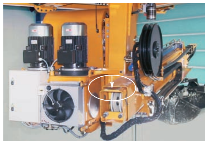
Sliding plates made of NYLATRON® 703 XL
