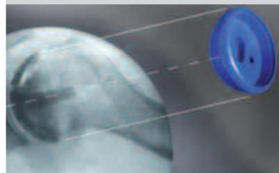
A contrast medium renders the APSOplast® material PPSU P MT XRO (TECASON P MT XRO) impervious to x-rays. That is why, for example, instruments or orthopedic test implants made from this material can be distinctly seen by surgeons with the help of imaging systems. The exceptional resistance of the plastic to strain caused by conventional sterilization techniques offers additional security.
