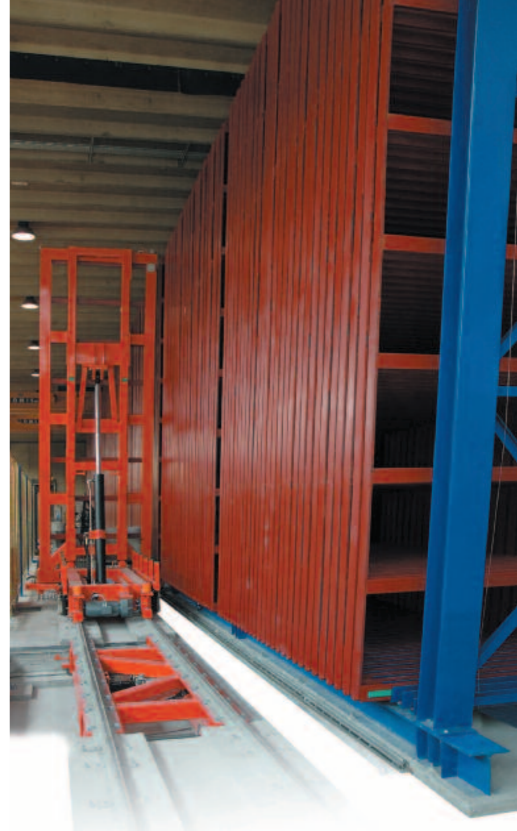
View of warehouse with movable frames mounted on the load-bearing structure of the fixed rack
