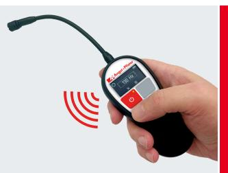
The correct pre-tension force has a significant influence on the operating behaviour and lifetime of the entire belt drive. It is one of the very few measurement variables that can be set by the operator himself. That's why it is highly recommended to set and check the pre-tension force of the belt with the TMconnect belt tension measuring device.
