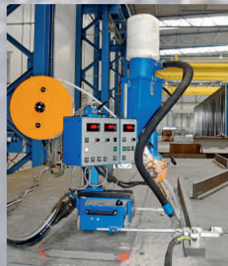
Mobile submerged arc welding tractor unit, view of carriage
