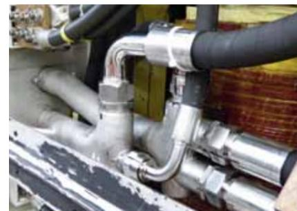
Connection of multiple electrical-converter cooling hoses
