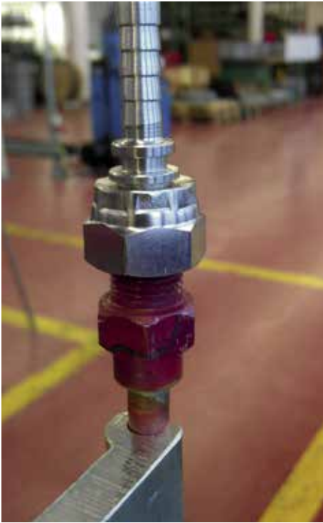
The connector fittings for the coolant lines are guaranteed leak-tight, as initial tests show.
