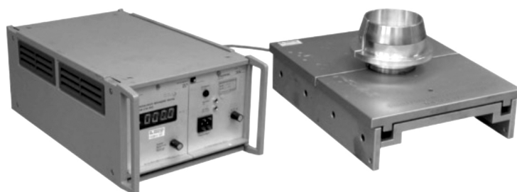
Exhibit 42 – Radial Force Measurement device acc. DIN 3761-9
