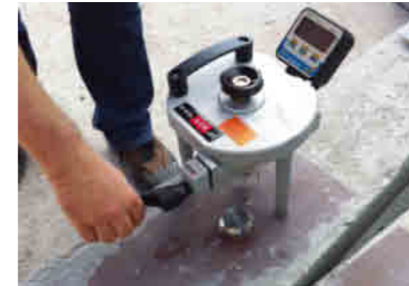
Pull-out test process.
