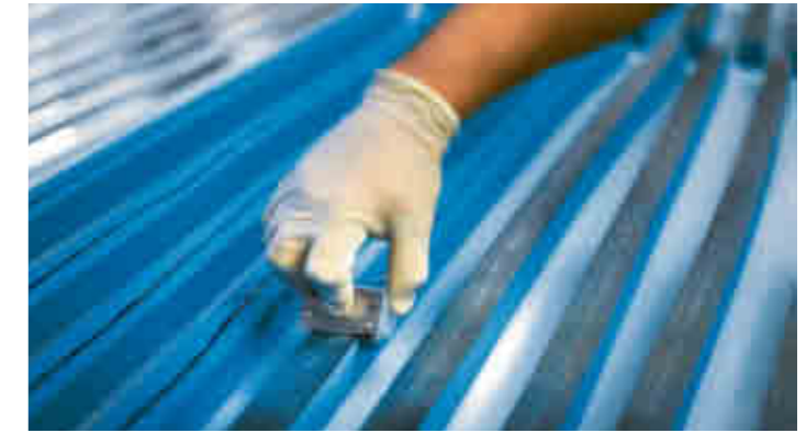
An aluminum plate is bonded to the polyurethane blocks. The adhesive bond is just as safety-relevant as the elastomer itself.
