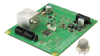
Figure 2. FCX-MC25-FLOW-A-CH OEM oxygen sensor module developed for in-line controlled atmosphere applications
