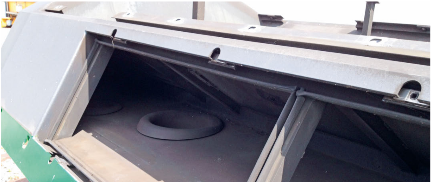
For maintenance the roof of the locomotive is removed. The original sealing frame for the filter grilles is clearly visible. It was cut to the correct length and glued to the corners.
