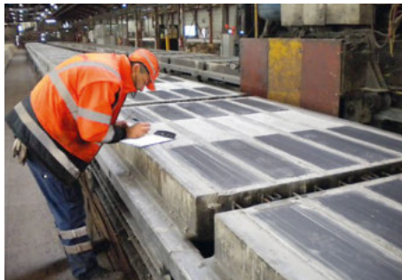
ECOVIB® USP sleeper pads: the special friction-fit method.
