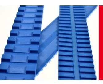
The BRECOprotect product line is specifically designed for the food and pharmaceutical industry. BRECOprotect are timing belts with steel cords completely enclosed in polyurethane, to protect them against corrosion.
